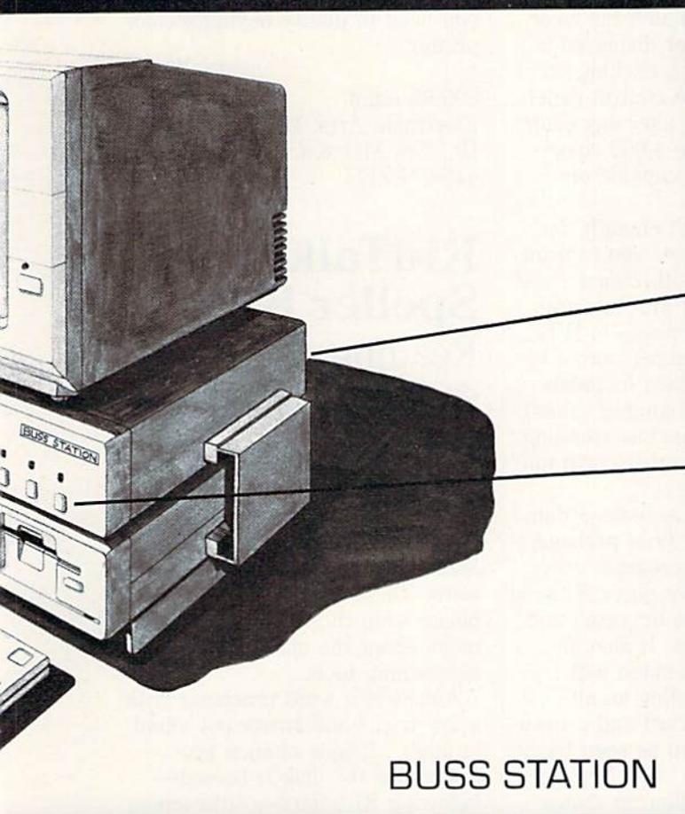
A special RAM expansion port which allows the user to plug in the DSI "Smarts" and incrementally increase the memory of the Amiga to its maximum potential of 8 megabytes.
